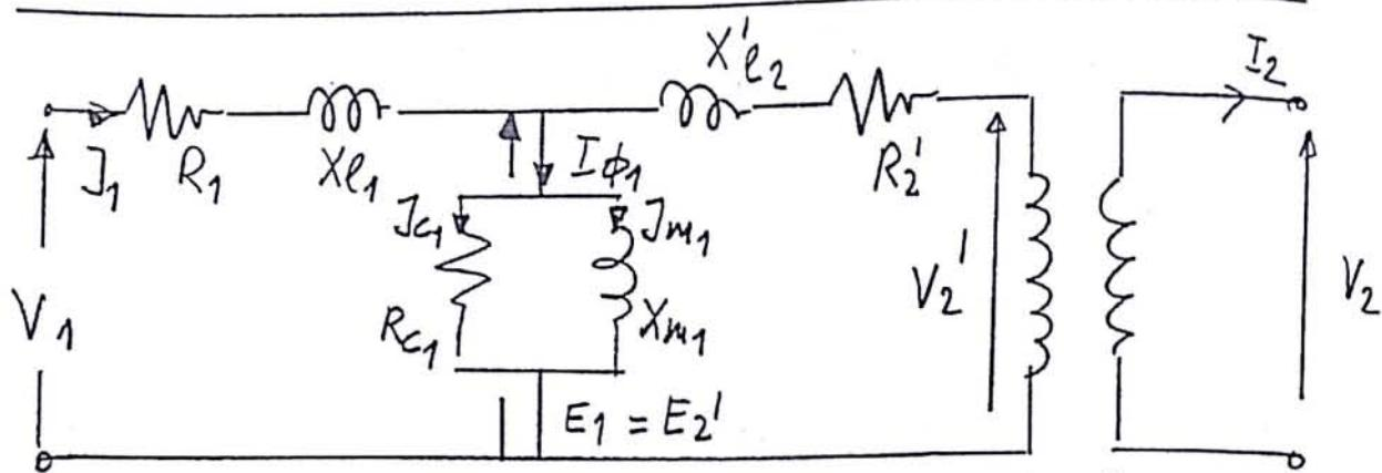
$$E_1 = E_2' = a E_2 \quad X_{l2}' = a^2 \cdot X_{l2} \quad \text{ideal transformator}$$
